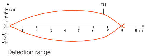
Retroreflective sensor with polarization BOS 21M-A-PR10
