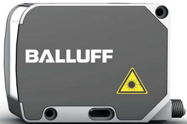
Optical distance sensors are used when distances of objects need to be measured or monitored with precise position determination. Distance measurement is based on either the triangulation principle or time of flight. PSD elements or CCD arrays are used for the receiving elements, with the emitter consisting of a red light or laser light source. Analog current and voltage values, serial interfaces and digital outputs are available to the user.
