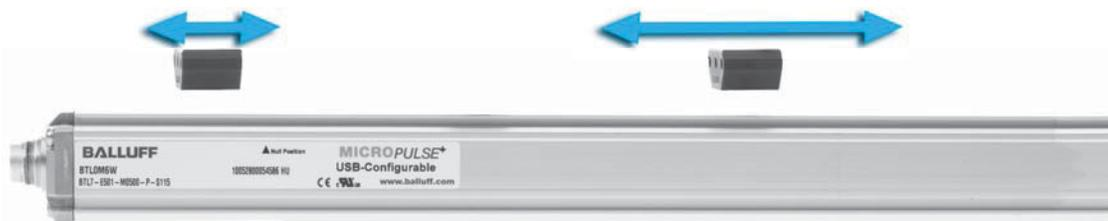
Micropulse+ position measuring systems guarantee cost-effectiveness and quality in the manufacture of concrete blocks. In a concrete block machine, the Micropulse+ position measuring system simultaneously and reliably measures the axis position of load and molding stroke movement.
