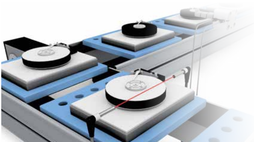
Precise height control of hard drives in an assembly line
