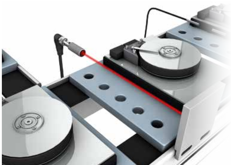
Detecting loaded pallets in an assembly line for hard drives
