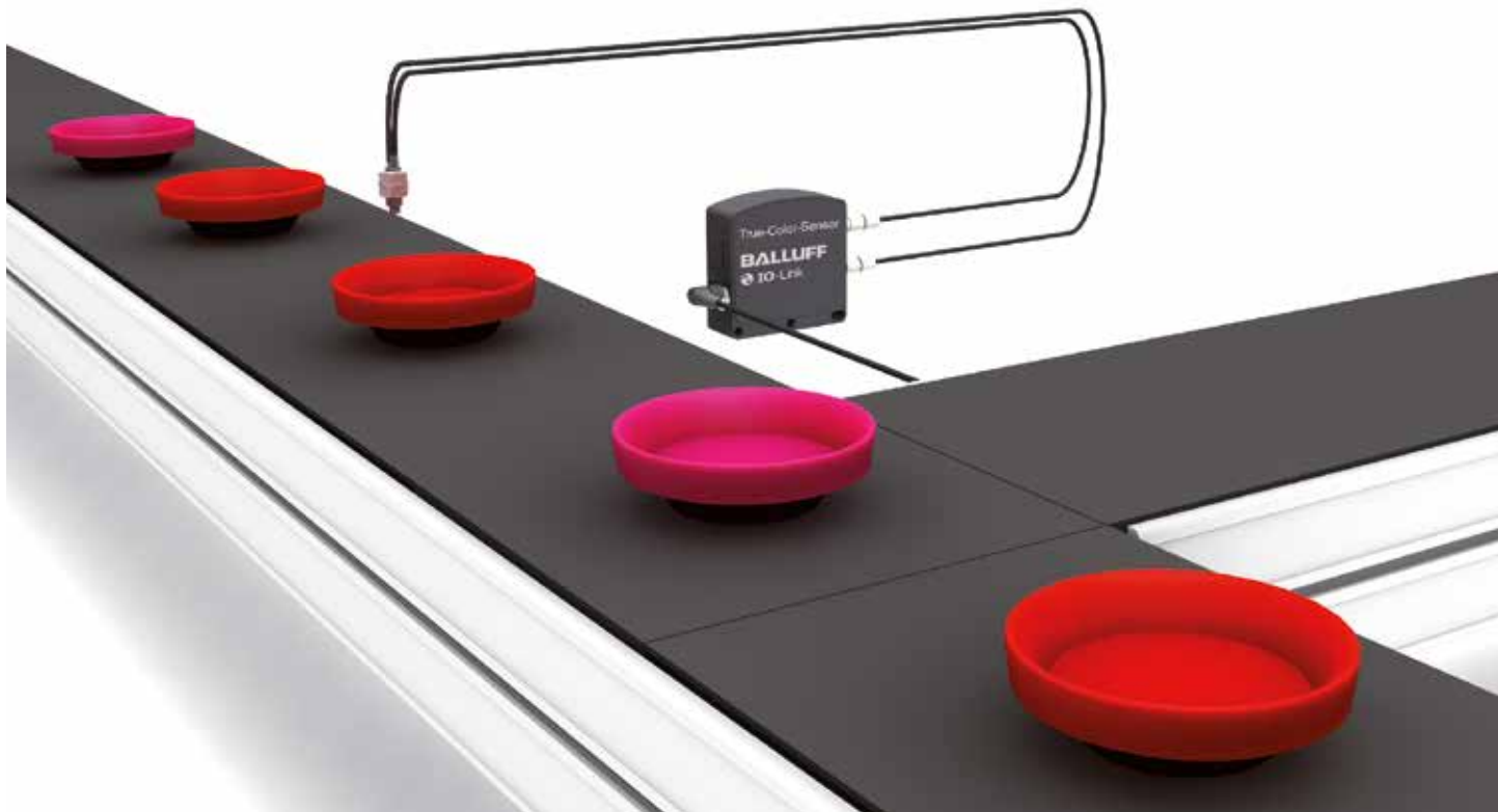
Plastic parts having slight color deviations can be reliably detected and quickly separated out.
